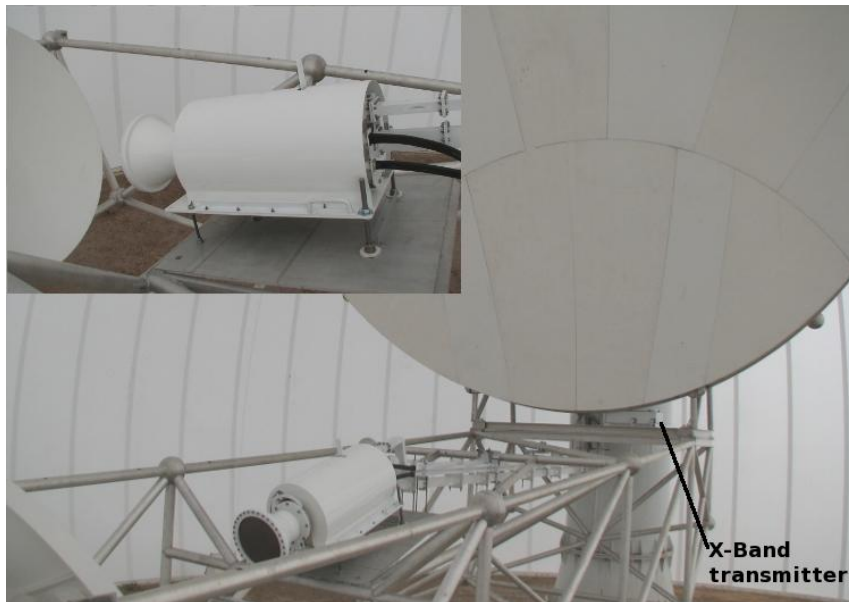
Figure 11: Dual frequency feed horn (inset) and X-band transmitter hardware installed on the CSU-CHILL offset antenna.
